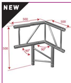
AGDU0-07 Corner joint - 3 directions - 45° - upright
